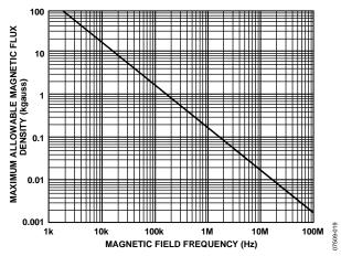
Figure 15. Maximum Allowable External Magnetic Flux Density
