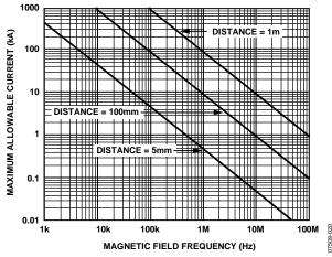
Figure 16. Maximum Allowable Current for Various Current-to-ADuM5400 Spacings
