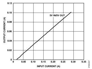
Figure 6. Typical Isolated Output Supply Current, I<sub>ISO</sub>, as a Function of External Load, No Dynamic Current Draw at 5 V/5 V
