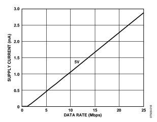
Figure 11. Typical I<sub>ISO(D)</sub> Dynamic Supply Current per Output (15 pF Output Load)
