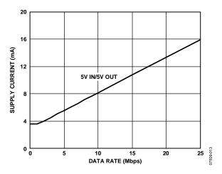
Figure 12. Typical I<sub>CH</sub> Supply Current per Forward Data Channel (15 pF Output Load)
