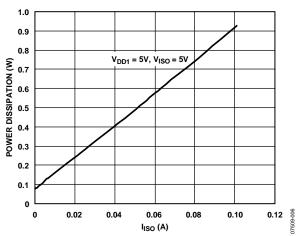
Figure 5. Typical Total Power Dissipation vs. I<sub>ISO</sub> with Data Channels Idle
