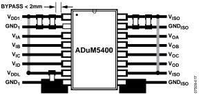
Figure 13. Recommended PCB Layout
