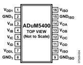
Figure 3. Pin Configuration
