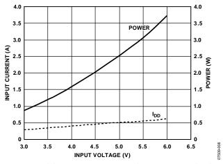
Figure 7. Typical Short-Circuit Input Current and Power vs. V<sub>DD1</sub> Supply Voltage
