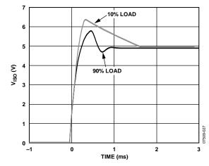
Figure 9. Typical  $V_{ISO} = 5 V$ , Output Voltage Startup Transient at 10% and 90%  $I_{Oad}$
